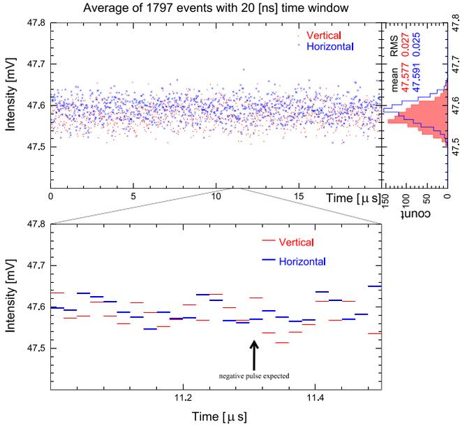
**Fig. 9.** Average waveform of the integrated intensity in a 20 ns time window over 1797 events. Signals from ten neighboring samples were integrated for each 2 ns sample. Positive 32.4 ns wide pulses starting at 11.31  $\mu\text{s}$  were expected. No signal can be seen in this measurement.
