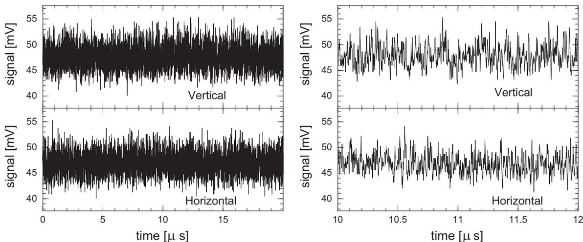
Fig. 8. Typical output-signal waveform from the power detector, as measured by the oscilloscope. Vertically and horizontally polarized signals were measured. The left panels show a  $20 \mu\text{s}$  long waveform and the right panels show the same signal but from 10 to  $12 \mu\text{s}$ . A negative pulse from 11.31 to  $11.34 \mu\text{s}$  was expected. No clear pulse was observed.
